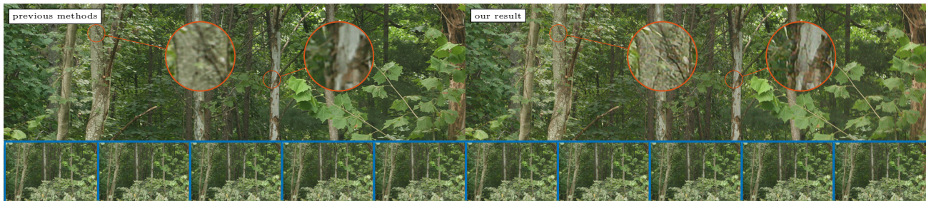
Figure 1. From a sequence of blurry inputs (lower row) our learning-based approach for blind burst-deblurring reconstructs fine details, which are not recovered by recent state-of-the-art methods like FBA [6]. Both methods feature similar run-time.
